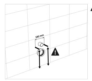
Please note, that the installation requires a pre-installed concealed cistern that must comply with standard EN 14055:2010. Leave enough space between the floor to tighten the bolts.
