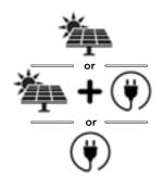
As soon as the battery falls below a specified voltage to maintain operation, the electronics automatically switch to mains operation. The battery is charged purely via the solar panel.
